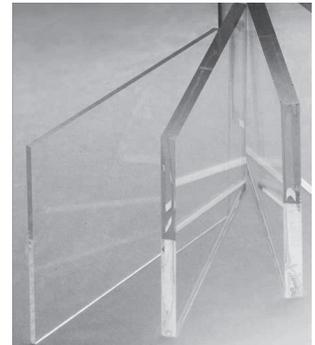
Pilkington Glass with silver plating of  $\geq 700\text{mg/m}^2$  ensures  $\geq 85\%$  reflectivity
